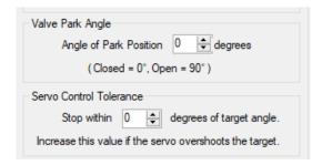
The Servo Control tab is used to set the closed and open positions. The valve can be driven continuously to the closed position or open positions, or nudged in small movements. Click and hold 'Drive in closed direction' and 'Drive in open direction' to drive the valve to the closed and open positions, respectively. Please check the Mk8 MM manual for further details.
