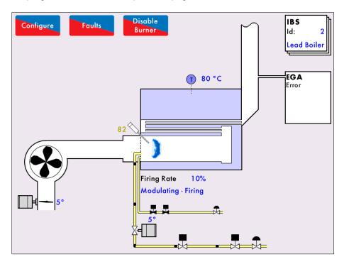
If the input range drops below 4mA or 0V an error will be displayed on the EGA screen.
