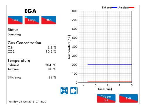
The exhaust gas temperature is related to input 2 on the interface, using a 4-20mA or 0-10V signal. The ambient temperature is taken from input 3 or the default value that is entered when setting up the interface on the PC.
