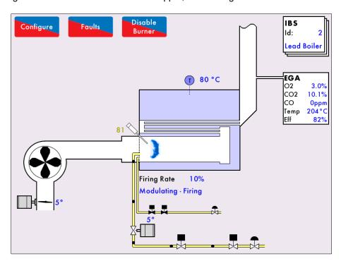
When burning natural gas, the CO<sub>2</sub> value is calculated to be approximately 10% when the O<sub>2</sub> is 3%.
