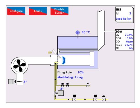
O<sub>2</sub> reading shows 20.9% when the 4-20mA or 0-10v signal is maximum (20mA or 10v). The efficiency reading will remain 0% until the O<sub>2</sub> reading is below 19%.
