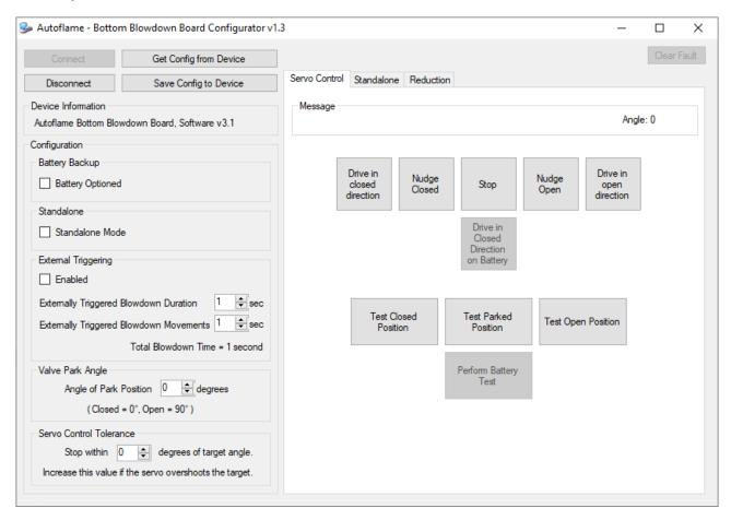
Check the tick boxes for 'Battery Backup', 'Standalone' and 'External Triggering' as required. External Triggering is used for when there is an external switch for the timed bottom blowdown trigger (see section 5.3.2). Please set the Valve Park Angle according to the bottom blowdown valve being used. For the Autoflame valves, this should be set at zero degrees.
