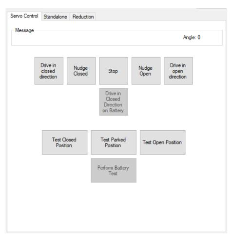
Once the open and closed positions have been set, these must be tested individually, by clicking 'Test Open Position', 'Test Closed Position', and 'Test Parked Position.'
