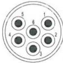
Figure 2.1.ii Mains Connector – Insert Pin Mating View
