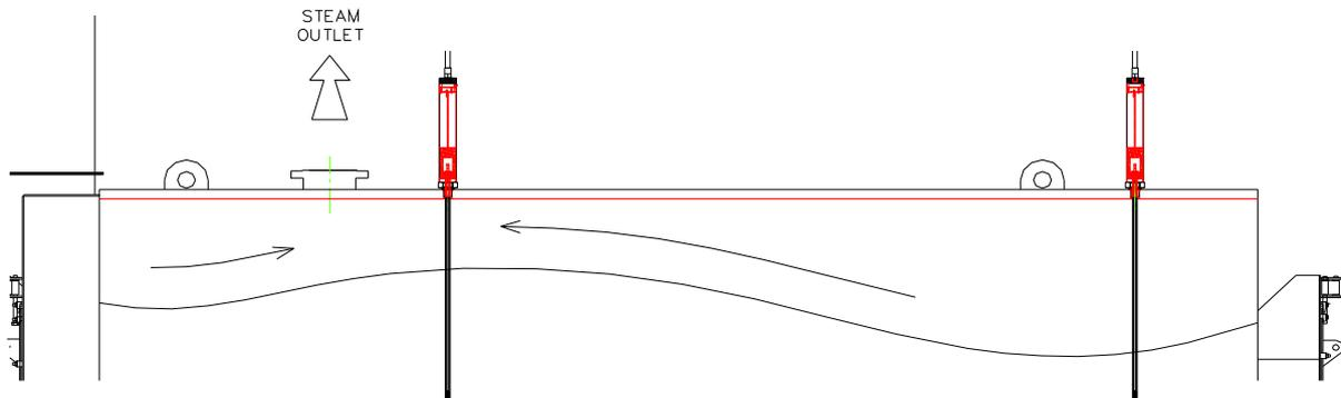
The above situation will be shown in high relief when the steam outlet is at one end of the boiler and one level probe is sited adjacent to the steam outlet and the second probe is sited at the opposite end of the boiler. The user adjustable probe disparity value may have to be increased to take this situation into account.
