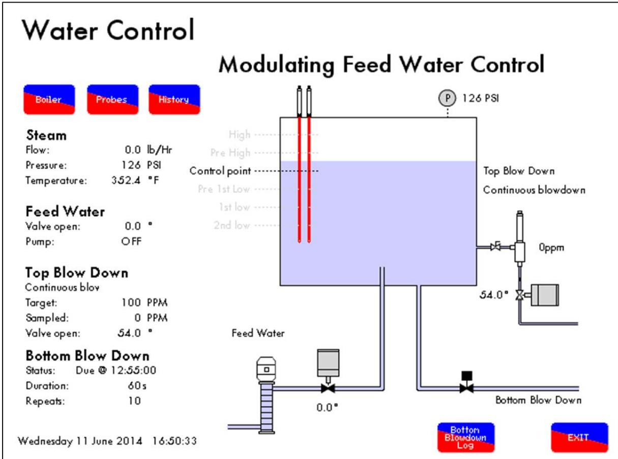
Figure 4.3.ii Water Level Screen
