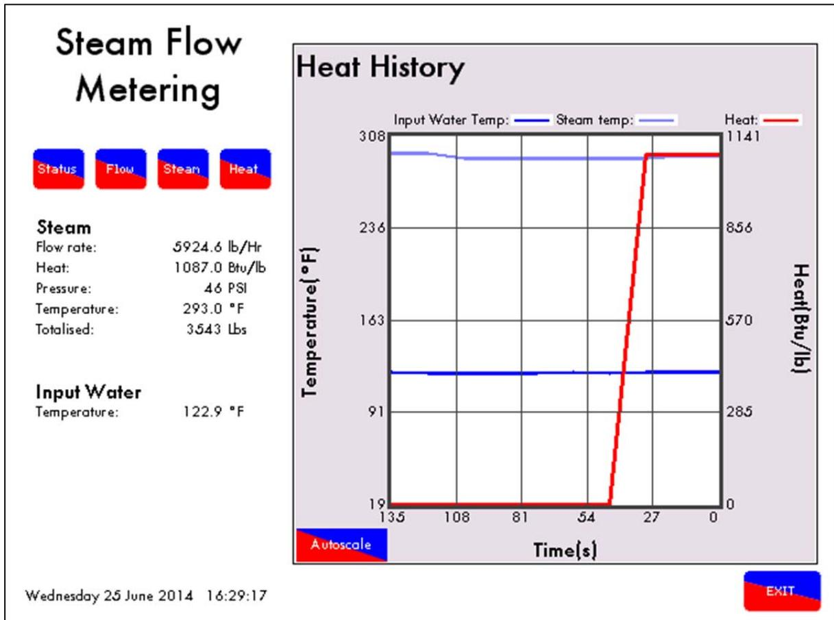
Figure 5.1.v Steam Flow Metering Heat History
