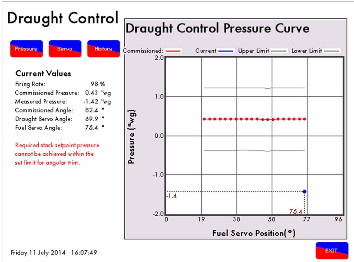
Figure 1.2.2.v Pressure Not Maintained
