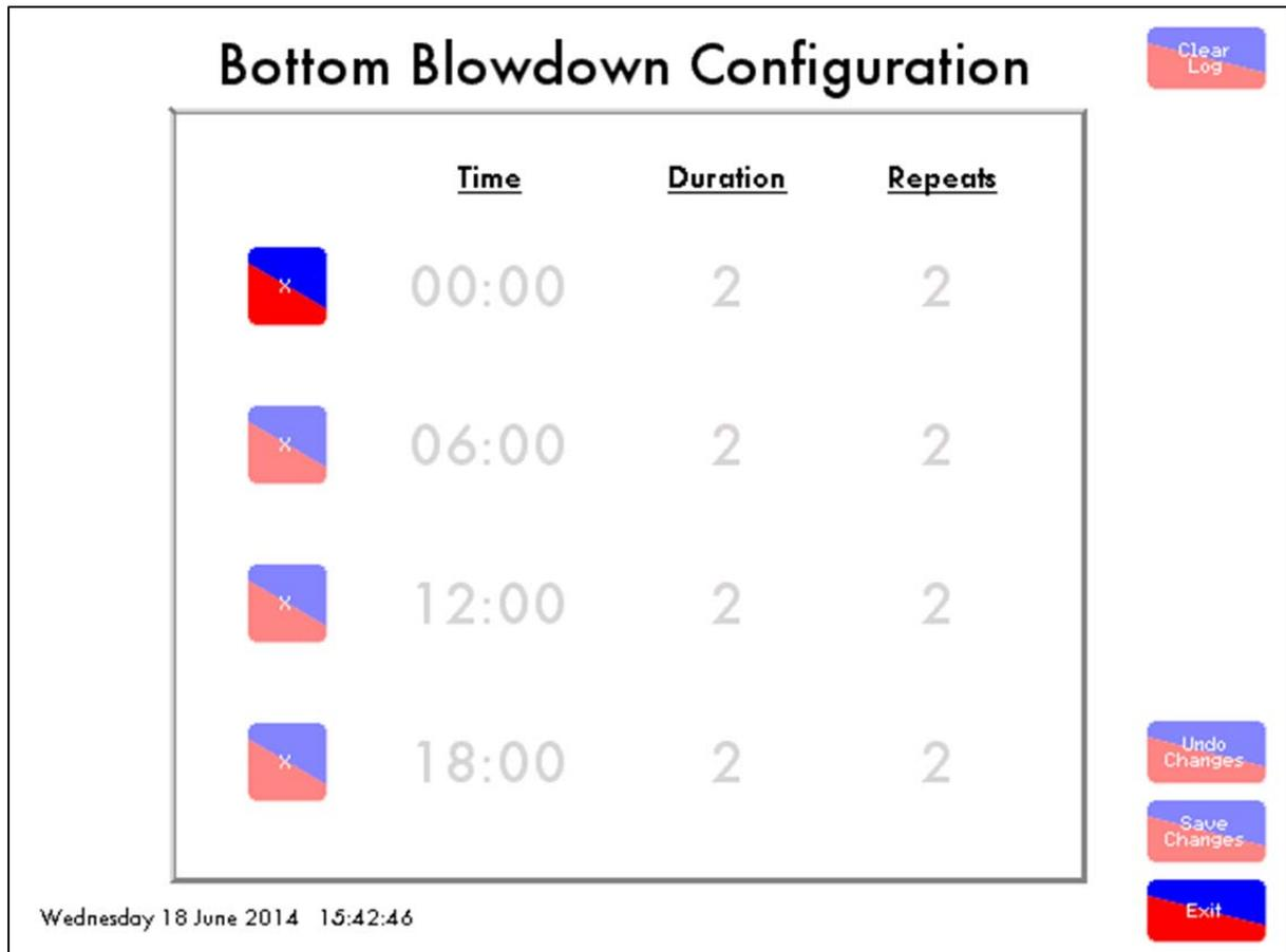
Figure 4.2.ii Bottom Blowdown Configuration Screen
