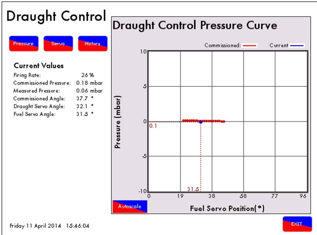
*Figure 1.2.2.ii Draught Control Pressure Curve*
