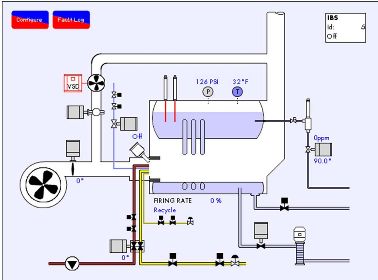
Figure 4.3.i Boiler Screen
