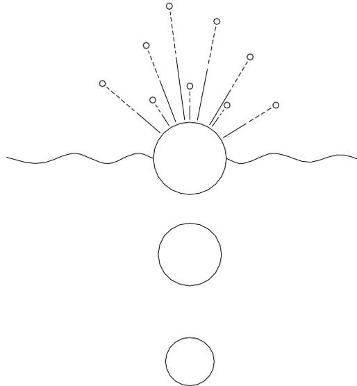
The droplets tend to coat the surface of the level probe which in turn will read as an increase in the water level. This situation is largely avoided by fitting anti surge pots inside the boiler shell. When the probes are fitted externally to the boiler shell this situation can not arise.
