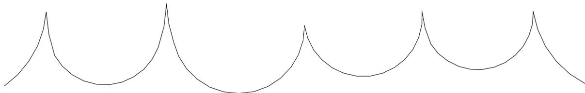
A second set of turbulence is the wave reflections off the sides of the boiler. The whole of the above is largely attenuated away by mounting the probes externally to the main boiler shell in a separate pot or pots.
